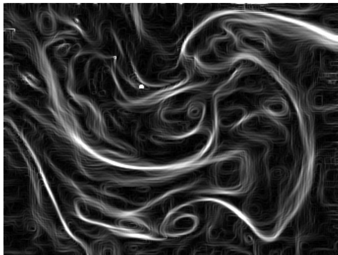
Figure. Sample of the scalar turbulent field. LIF measurement [1].
